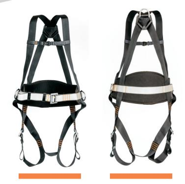
This 3-point harness combines simple and ergonomic harness with comfortable work positioning belt, two-inone. The harness id fitted with a rer D-ring and two side D-rings mounted to the belt for pole climbing or can also be used for work positioning on various open structures.
